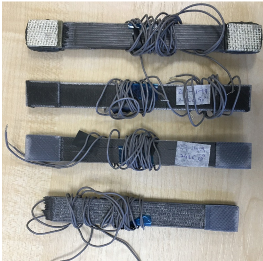
Fig. 9. Rectangular tensile samples with 3D printed and glass tabs with strain gages.
