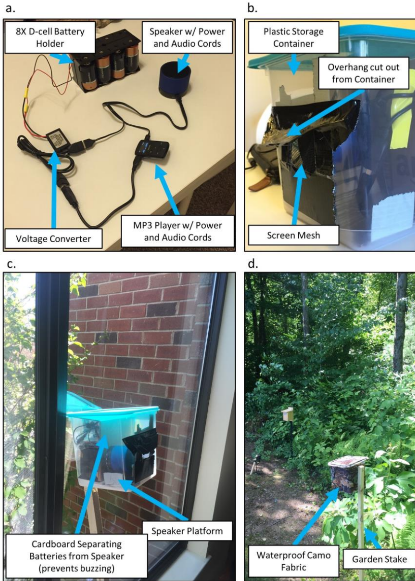
Figure 15. Schematic diagram of portable playback speaker unit assembly. (a) Shows internal electrical components along with (b) container, (c) mount, and (d) set up in situ. Portable playback speaker units last approximately 3.5 days with 8 rechargeable D-cell batteries and audio playing at our calibrated amplitude, rates, and duration. Speaker units were rotated every 3 days.
