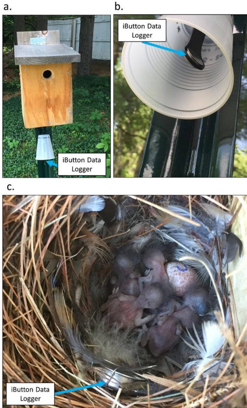
Figure 18. iButton temperature loggers were placed both external and internal to nests. (a) Suspended plastic cup containing hanging external iButton, (b) external iButton suspended by wire filament, and (c) internal iButton wired into side of nest cup (exposed for visibility).
