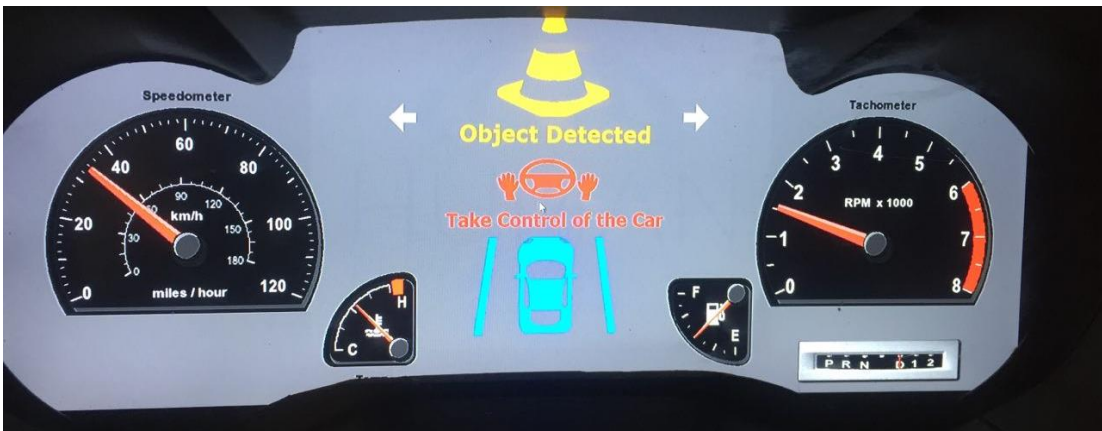
Figure 14. Advanced Dashboard showing an intersection ahead (Fourth iteration)
