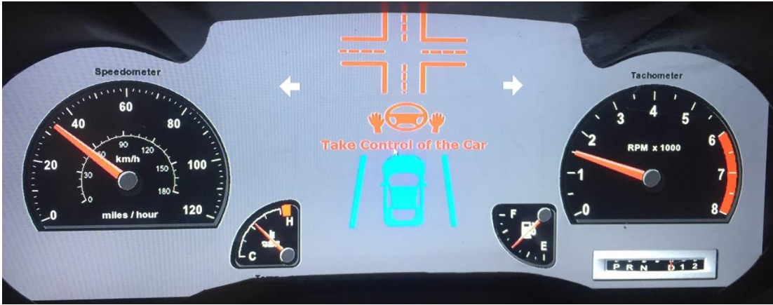
Figure 14. Advanced Dashboard showing an intersection ahead (Fourth iteration)
