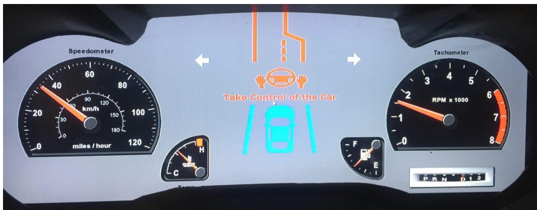
Figure 12. Advanced dashboard showing the object detected icon (Fourth iteration)
