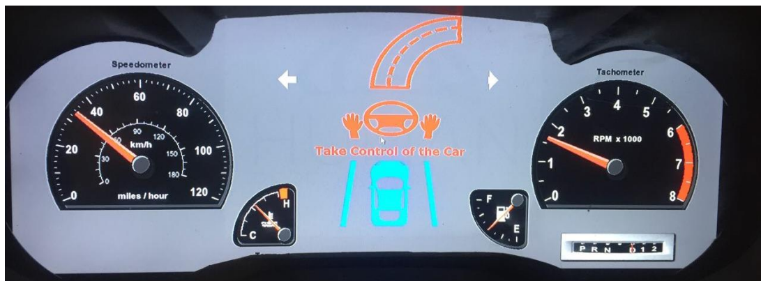
Figure 13. Advanced Dashboard showing a curve ahead (Fourth iteration)
