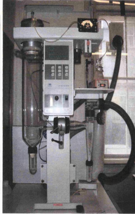
Figure 3.1: Schematic and photograph of Buchi Mini Spray Dryer 191, where A = feed pump tubing, B = compressed air inlet, C = pneumatic nozzle, D = drying chamber, E = control panel, F = sample feed holder, G = cyclone, H = collection vessel and I = aspirator (Buchi, 2002).
