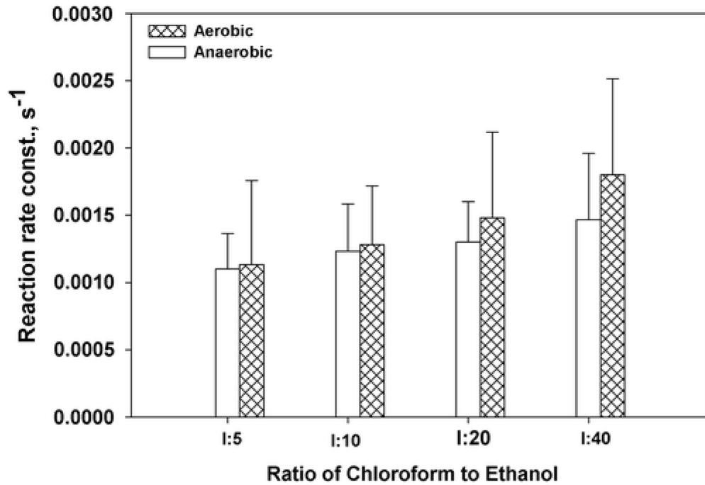
**FIG. 3.** Reaction rate constants for chloroform for both anaerobic and aerobic BTFs in the four phases. Phase I: 1:5, phase II: 1:10, phase III: 1:20, and phase IV: 1:40 chloroform to ethanol.
