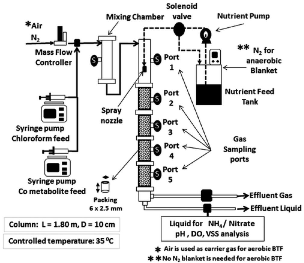
FIG. 1. Schematic diagram of anaerobic and aerobic BTFs. BTFs, biotrickling filters.
