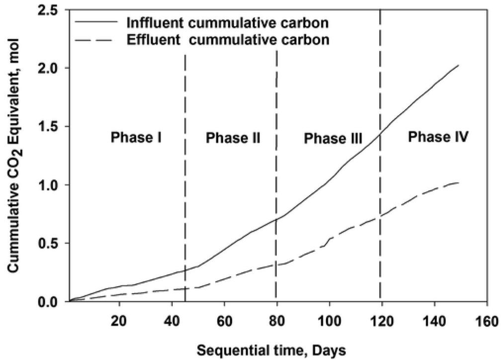
**FIG. 4.** Carbon mass balance: cumulative carbon input and output as CO<sub>2</sub> equivalent in mole for anaerobic BTF. CO<sub>2</sub>, carbon dioxide.
