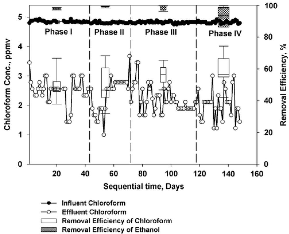
**FIG. 2.** Performance of anaerobic BTF in four phases. Phase I: 1:5, phase II: 1:10, phase III: 1:20, and phase IV: 1:40 chloroform to ethanol. The *box* and *whiskers* plot show the median removal efficiencies and quartiles of  $\text{CHCl}_3$  and ethanol for each operation phase.
