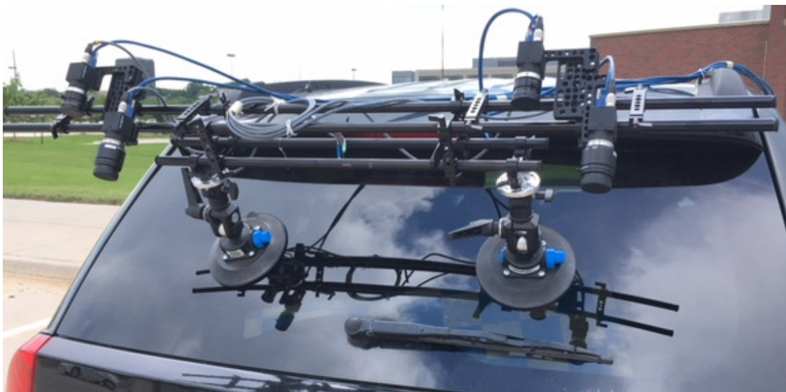
Figure 2. Multi-view camera system mounted on a road vehicle.
