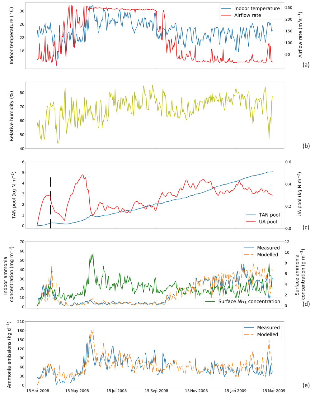
Figure 4. Site simulations using a fixed resistance ( R^* ) value of 16\,700\text{ s m}^{-1} for House A at site NC2B, Nash, North Carolina, from 15 March 2008 to 15 March 2009. (a) Measured daily mean indoor temperature and airflow rate of the house. (b) Measured daily mean relative humidity of the house. (c) Modelled TAN pool and UA pool. The black dashed line indicates the house-emptying date of 9 April 2008. (d) Comparison between measured and modelled indoor \text{NH}_3 concentrations of the house and surface \text{NH}_3 concentrations. (e) Comparison between modelled \text{NH}_3 emissions and calculated \text{NH}_3 emissions from measured indoor concentrations. The simulation illustrated uses the new parameterization (based on the AFO data; Fig. 3) for the relative humidity dependence of UA hydrolysis.
