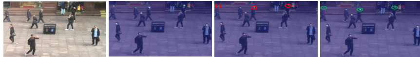
Fig. 3. Qualitative example of density maps. From left to right, the columns correspond to a cropped input video frame from the FDST dataset [9], ground truth density map, density map from the proposed baseline (without optical flow), and the density map from the full MOPN model. Superimposed red and green circles highlight certain false negatives and true positives, respectively. Best viewed in color and with magnification.
