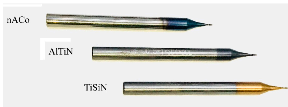
Figure 2. Different coated microdrill tools used in the experiments.
