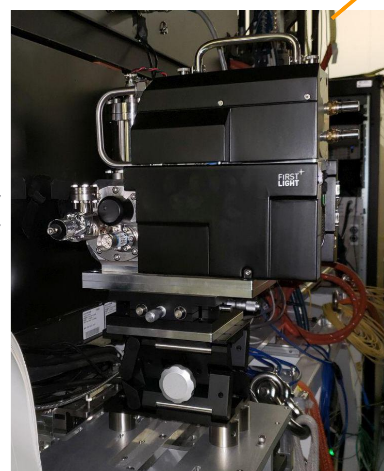
First Light Imaging C-RED ONE installed on the side of SCEXAO, where Ifa's custom SAPHIRA camera used to be for testing. In the future, the camera will also be able to use another port on the side of AO188, to be used as a NIR PyWFS.
