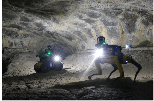
Fig. 1. Spot and Husky robots exploring a subterranean environment in Valentine Cave, Lava Beds National Monument, California. Obstacle avoidance in unstructured environments incurs higher mission risk due to lack of global positioning [9].
