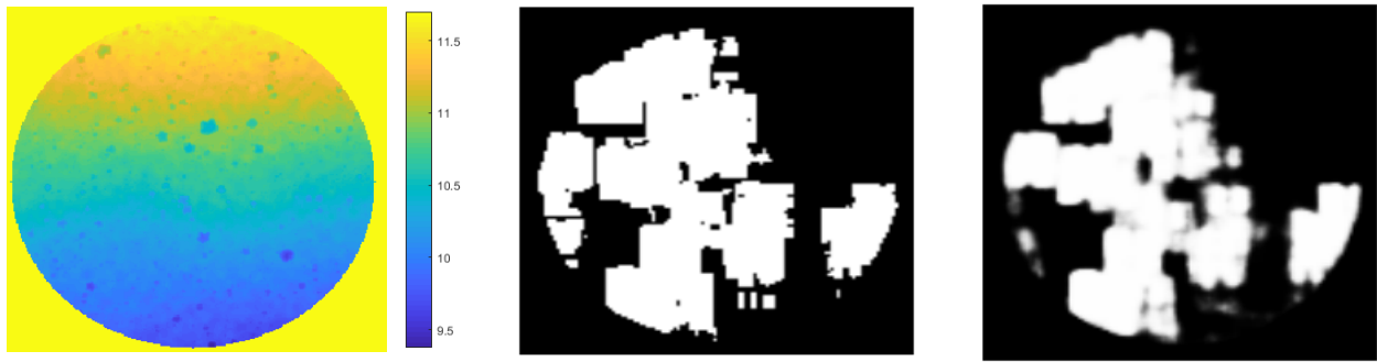
Figure 3: An example of a Learned Heuristic. Sets of terrain heightmaps (left) and maps generated by the ACE algorithm (center) were used to train a neural network to generate an inferred ACE probability map (right).
