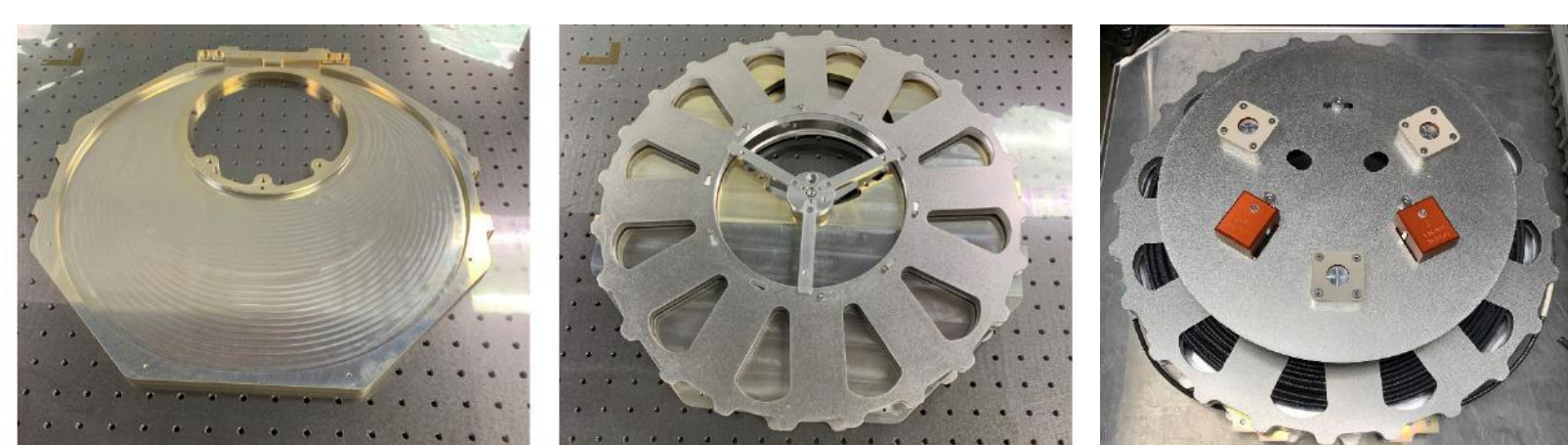
Left: Strain relief box (inside). Smaller circle is set at fiber minimum bend radius. Center: Miniflex storage spool mounted on strain relief box. Right: Strain relief box and spool in fiber AR-coating configuration.
