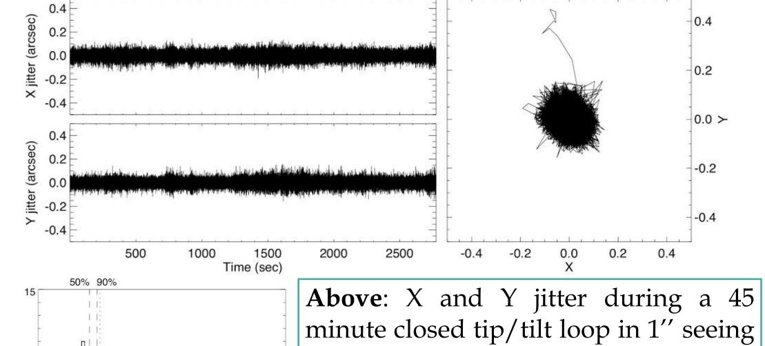
minute closed tip/tilt loop in 1" seeing using 2D cross correlation centroiding. **Left**: RMS performance for above data. In this run, 96% of one minute intervals showed≤50 mas motion, meeting our requirement.
