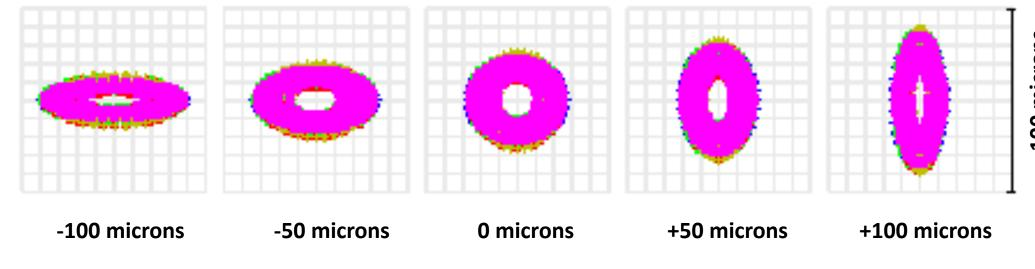
mirror focus Above: Zemax spot diagrams of our toroidal lens design. If our sweeps taken periodically through the target is in focus, the spot will be circular, otherwise the spot is elongated.
