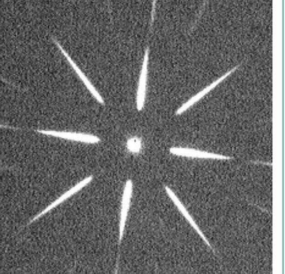
addition to our ADC prisms, the Port Adapter includes a Ronchi grating that is deployable in front of the guide camera (see on-sky image at left). Once fully commissioned, this grating will enable us to precisely calibrate the ADC by measuring and correcting for residual atmospheric dispersion similar to Pathak et al. (2016, 2018).
