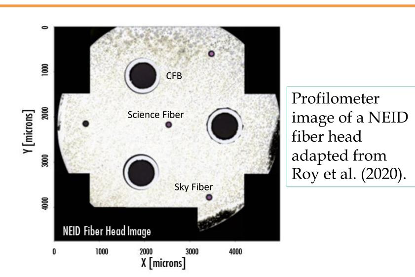
A dedicated assembly images the six NEID CFBs (3 from each Fiber Head). CFBs preserve spatial information over a larger FOV than a single fiber (5.6" vs 0.92" in HR fiber). The CFBs allow us to:
