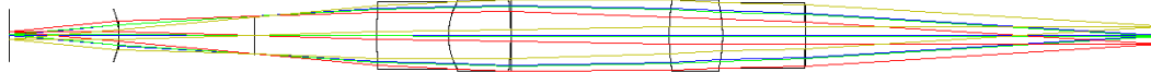
Figure 5. Glasses in the doublets are (N-BK10, S-FPL51Y) and (S-FPL53, NIGS5742). Shown is only the lens diameter at the clear aperture, which is 3.4mm.
