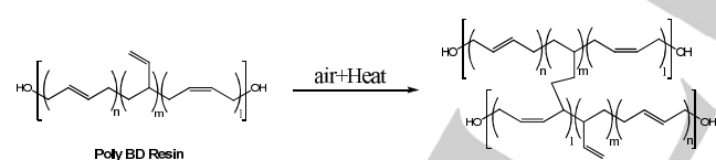
Figure 2. Self-cross-linking of the alkene groups in polybutadiene P6 (Poly BD R45HT-LO).
