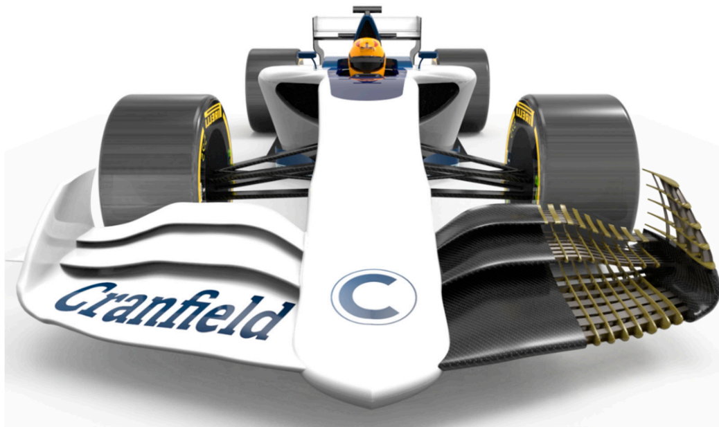
Figure 11. Selected structural components of the Formula One 2022 front wing.
