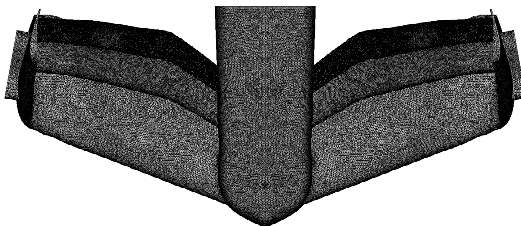
Figure 4. Mesh of the 2022 Formula One front wing assembly.
