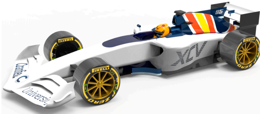
Figure 2. 2022 front wing attached to a 2018 Formula One car (the whole design is performed and developed by the authors).
