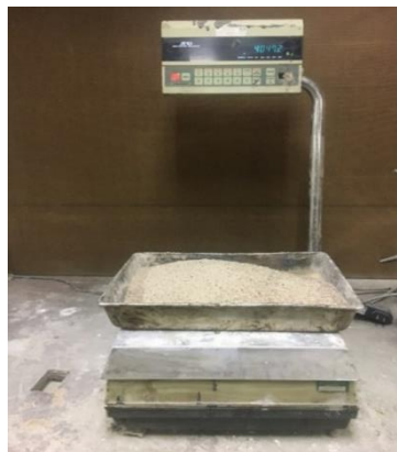
Figure 3.4. Weighing fine aggregate (sand)
