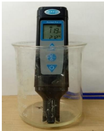
Figure 3.17. Measurement of pH value of pore solution
