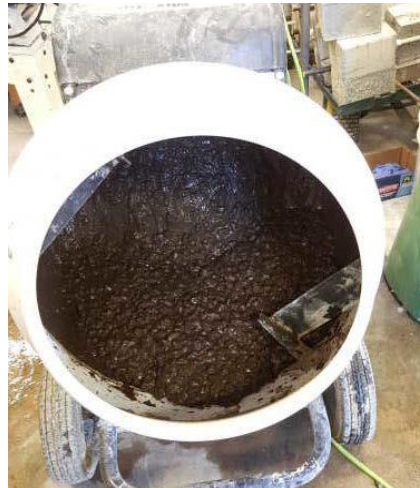
Figure 3.11. Mixing of geopolymer concrete
