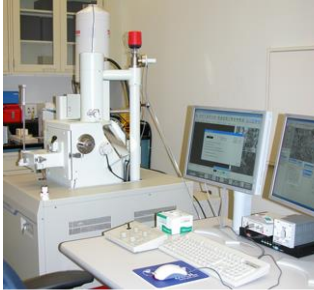
Figure 3.19. Scanning electron microscope
