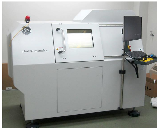
Figure 3.24. GE v|tome|x s microCT scanning device
