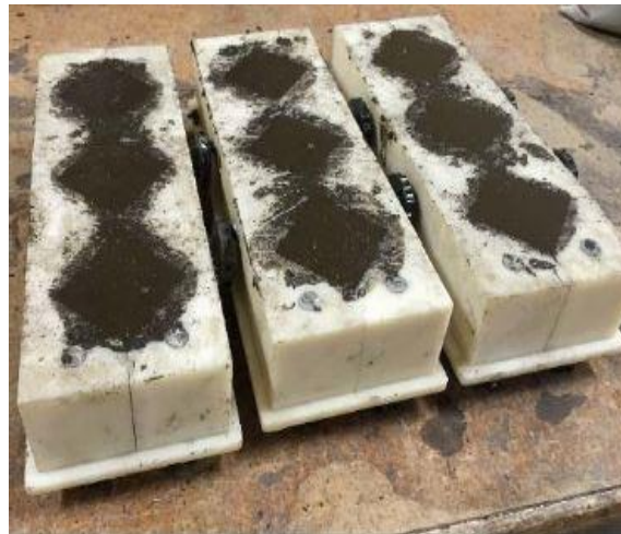
Figure 3.23. Molding of 2 x 2in concrete cubes
