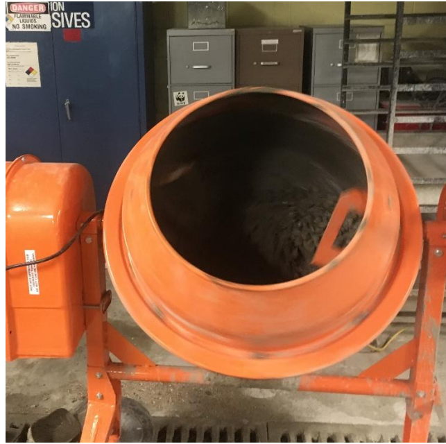
Figure 3.12. Mixing of OPC concrete
