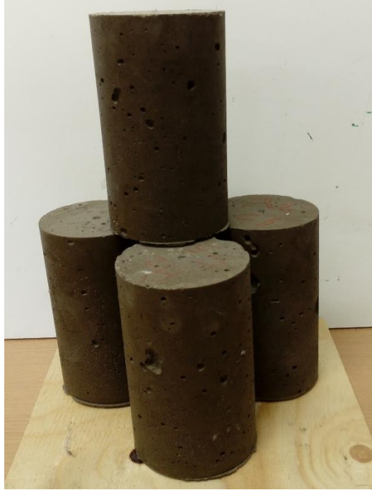
Figure 3.15. Geopolymer concrete cylinder specimens
