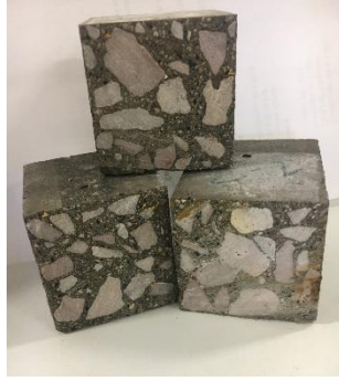
Figure 3.20. Cube specimen used to make slices for FTIR analysis
