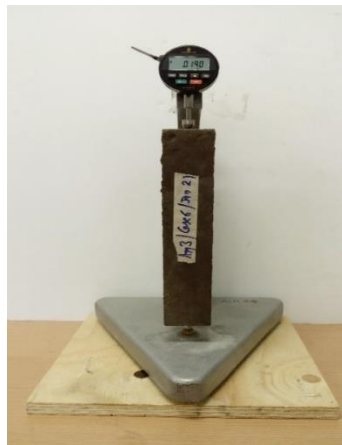
Figure 3.14. Length change measurement setup
