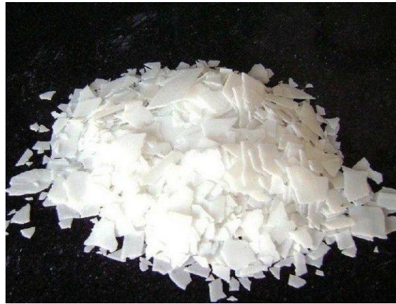
Figure 3.8. Sodium hydroxide flakes
