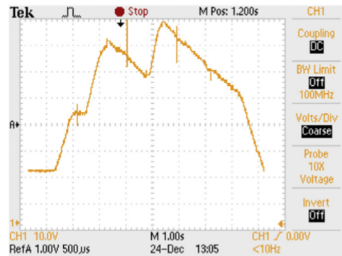
Fig. 1. Experimental output voltage waveform of the PV arrays under different environmental temperature and partially shaded condition.
