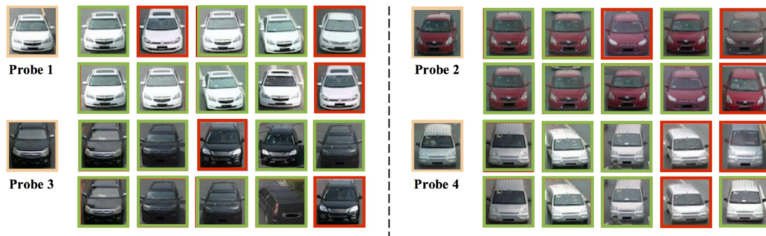
Figure 4.7: Four examples of vehicle re-ID results (Rank-5) on the VehicleID dataset. For each probe, the ranking results produced by our baseline are presented in the first row, the second row corresponds to our proposed method (Semi-supervised learning+re-ranking) which improves the baseline ranking results. The green box indicates a true matches, the red box identifies the false matches.
