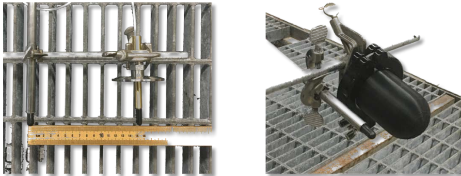
The picture shows the two hydrophones mounted in close proximity to compare their responses. Their output signals were recorded simultaneously.
