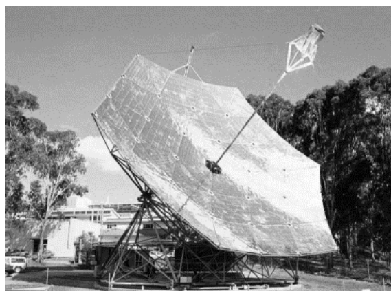
Figure 28. ANU ammonia synthesis system. Source: [25].
