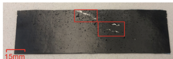
Figure 9. Defects on specimen: porosity (black features on the surface) and void (highlighted with red boxes).
