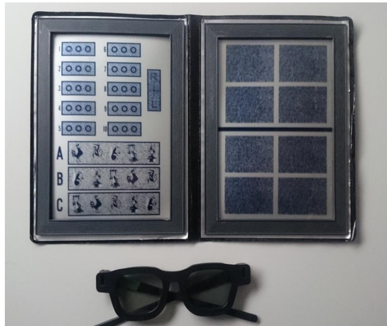
Figure 2.3. Randot Stereo test and the polarising filters through which each of the random dot stereograms in the right-hand plate were viewed. Observers reported the shape perceived in depth. In the left-hand plate animals or Wirt circles were at different disparities to indicate stereoacuity.
