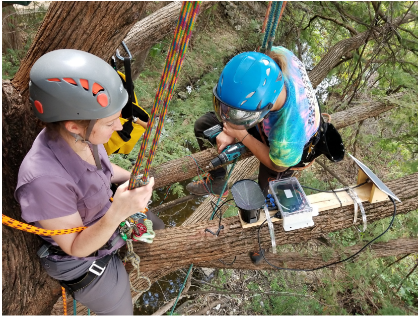
Fig. 10. Installed branch node. Sap flux sensor (left of the rain gauge) is shown without reflective covering to show detail.
