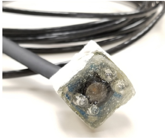
Fig. 4. Epoxy potted turbidity sensor.
