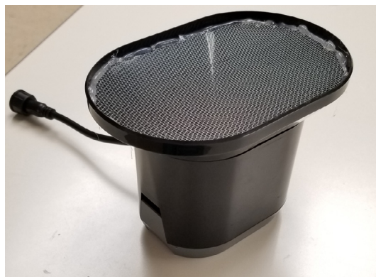
Fig. 2. Tipping bucket rain gauge shown with wire mesh cover and cable modification.
