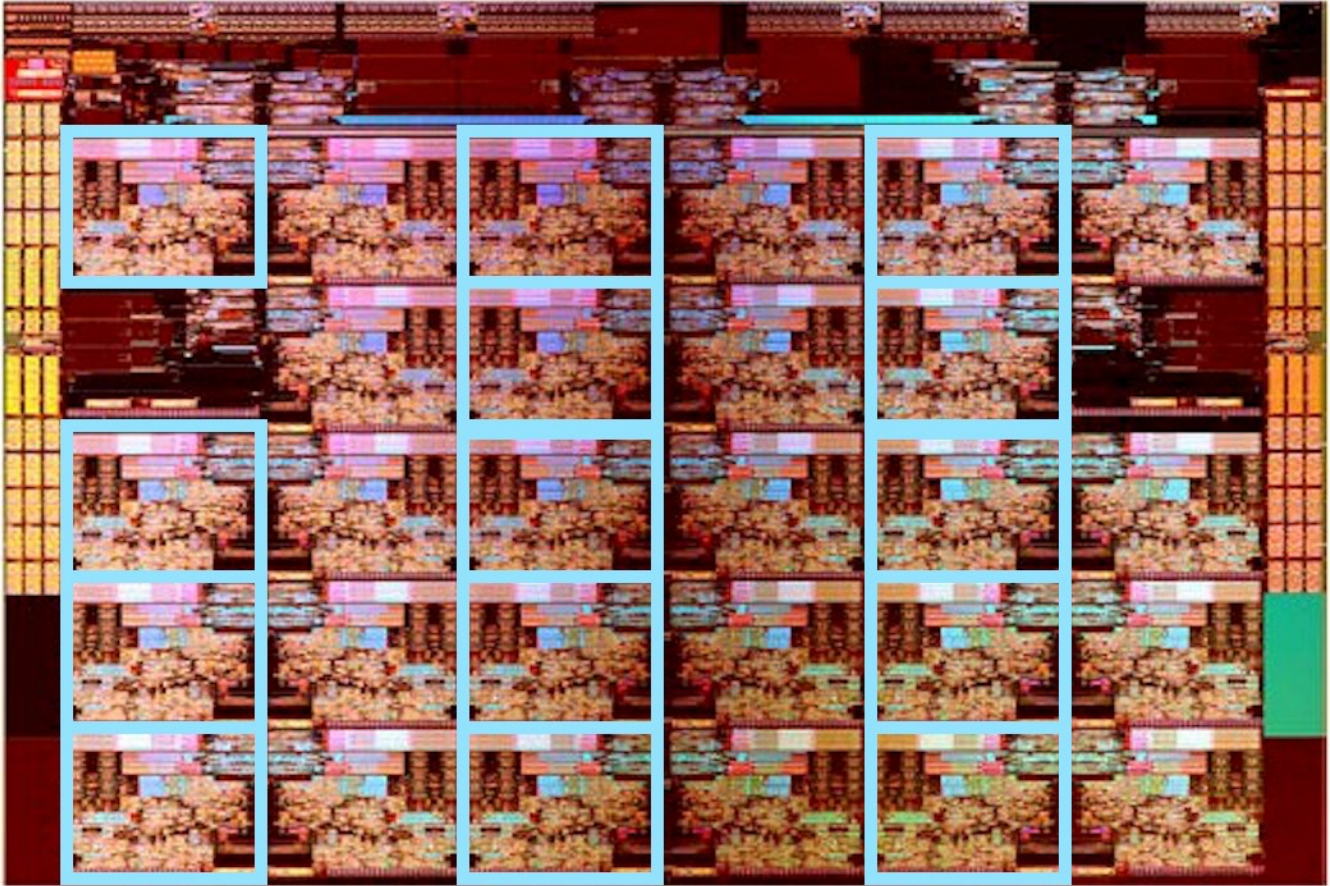
Figure 5: Die photo of the XCC (28-core) Xeon Scalable Processor. The cores in columns 0, 2, and 4 (outlined in light blue) are in the "standard" orientation, while the cores in columns 1, 3, and 5 are laid out with left-to-right mirroring. (Image from [4], annotations added.)
