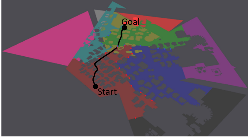
FIGURE 3.5: Example scenario, where connecting S and G becomes a bottleneck due to the large number of inter-edges .
