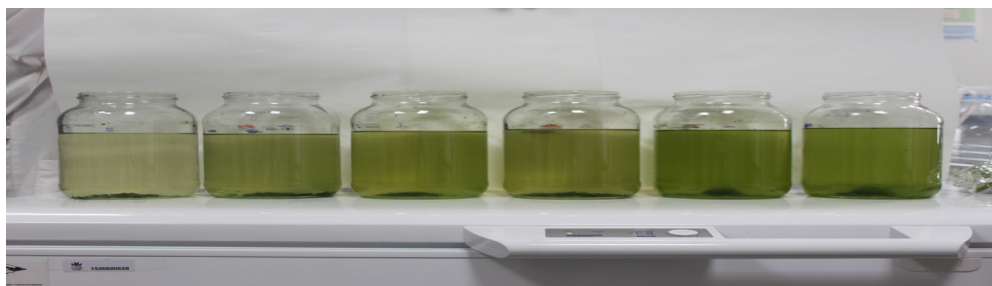
Figure 2. Reactors used in the experiment. From left to right in decreasing order of HRT.
