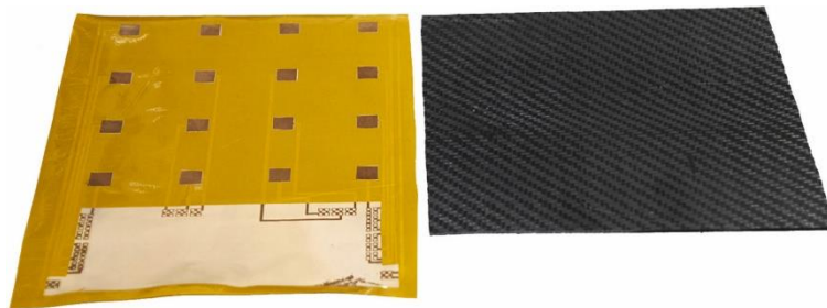
Figure 9: Flexible sensing mat (left) to be attached onto CFRP panels (right) [81].
