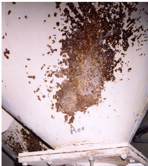
Fig. 2 “Hammer rash” on bins with flow problems – the effects on the bins are obvious, but how much damage has this done to the operators?
