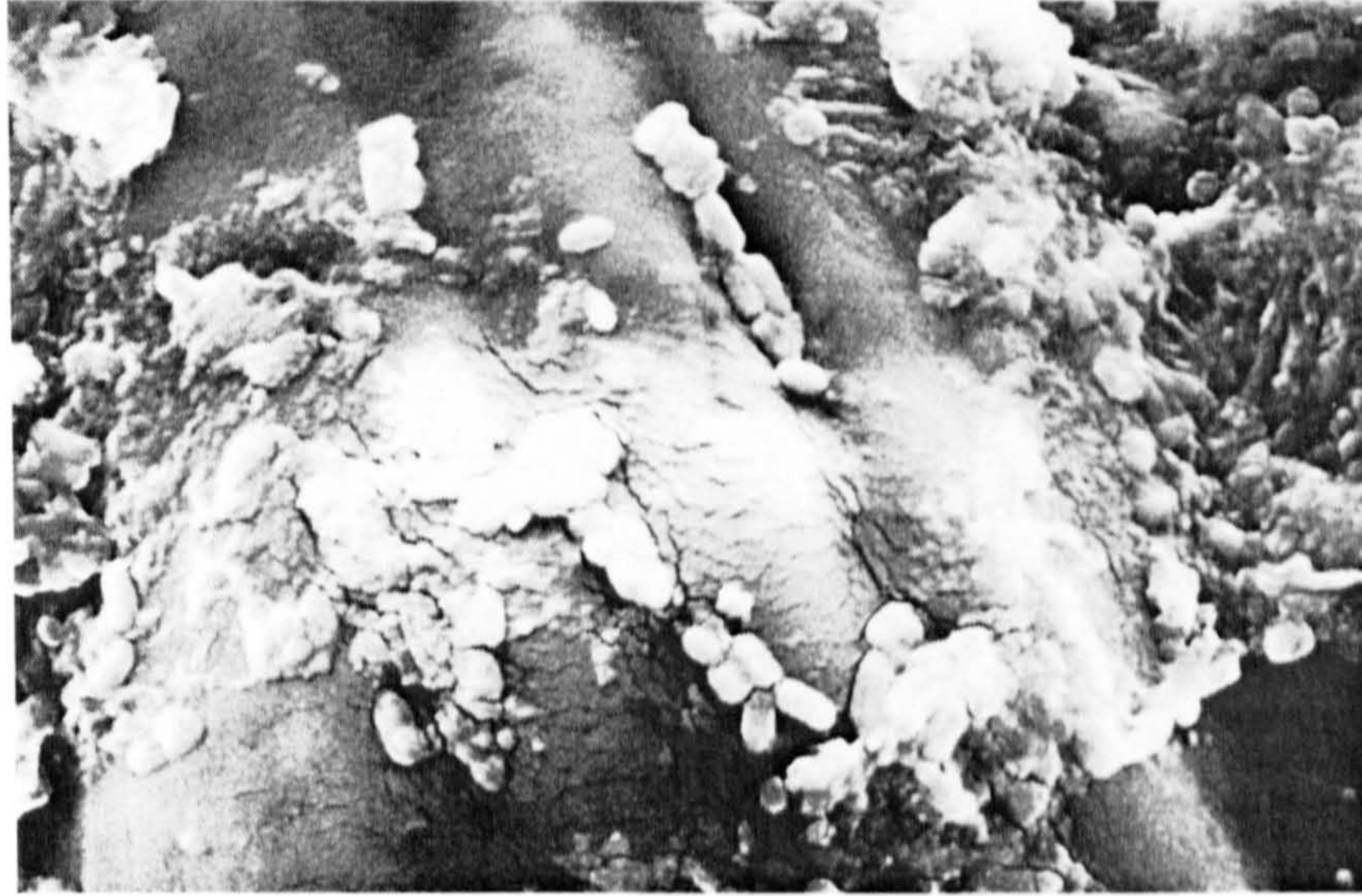
Fig. 5.55 Scanning electron micrograph of Nephrops shell waste subjected to lactic acid fermentation for 1 day (x2500).
