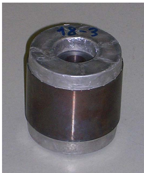
Fig. A2.5 Manufactured cast rotor
