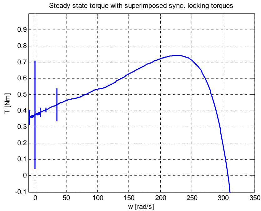
Fig. 6.6 Steady-state torque-speed curve with synchronous locking torques superimposed for 230 V motor and 18 rotor slots
