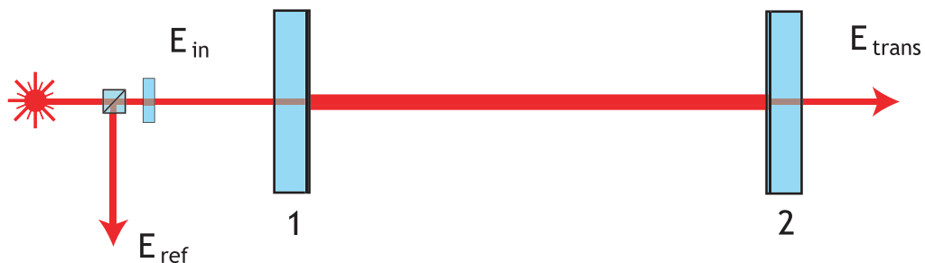
Figure 2.2: A schematic of a Fabry-Perot cavity. Mirrors 1 and 2 (with amplitude reflection and transmission coefficients \rho_1, \rho_2, \tau_1, \tau_2 ) are separated by a length L , with their reflective surfaces facing each other. The light reflected from the system is separated from the input light with a polarising beam-splitter and quarter wave-plate setup.
