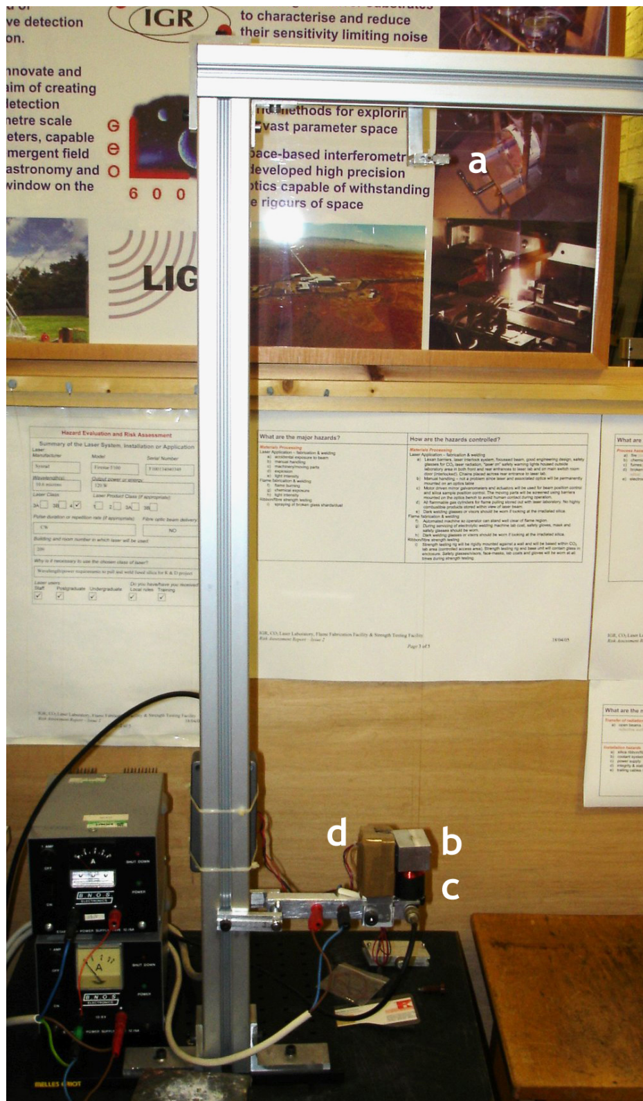
Figure 4.5: Apparatus for “bounce testing” the silica fibres, to determine their average diameter. Fibres were clamped at the upper stage (a), and attached to a free mass (representing the design payload) at the lower end – b. A magnet attached to this lower mass was then excited by a coil (c), driven by the voltage output of a signal generator. The frequency of maximum vertical response of the system could then be measured by observing the trace on an oscilloscope of a flag moving past a split-photodiode (d).
