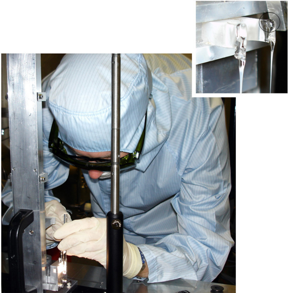
Figure 4.11: Test welding a silica fibre to an example ear. The fibre is first held in a tweezer jig, and manipulated using silica pieces as tools. The inset shows an example ear and the different stages of fibre welding: the area circled is considered monolithic, the area immediately below this is unfinished, and the near fibre is only attached via a placeholder weld.
