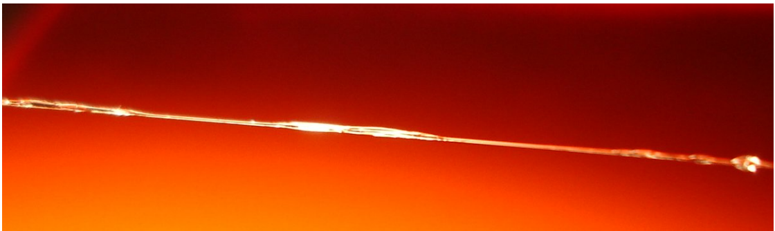
Figure 4.8: Detail of a test silica fibre, coated with damping material over three areas. Care had to be taken to ensure that the coating was as homogenous as possible and did not form unwanted globules – see the rightmost area.
