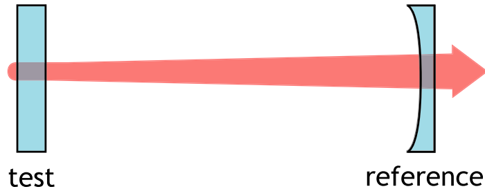
Figure 3.2: A schematic layout of a thermal noise measurement cavity: the input coupler is flat, with its reflecting surface coinciding with a beam waist. The end mirror is concave and more reflective than the input optic. The thermal noise contribution from the input mirror dominates the measurement.
