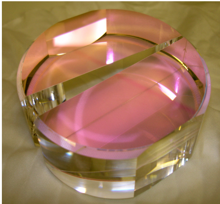
Figure 4.27: A replacement thermal noise experiment test optic. Here the optic is shown in two pieces, prior to silicate bonding. This will create a composite mass with the lossy bond layer close to the measurement beam, allowing the effect of the bonding process on the thermal noise spectrum to be directly quantified.
