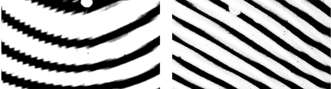
Figure 4.13: Interferometry measurement of the relative flatness of two sides of an upper stage mass. One side (the figure to the right) is seen to be polished to the requisite \lambda/10 , where the other side is only \sim \lambda/3 .
