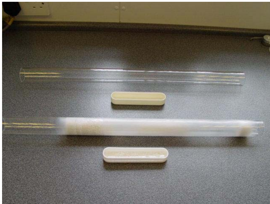
Figure 5: Quartz sleeve before (upper) and after (lower) the combustion stage
