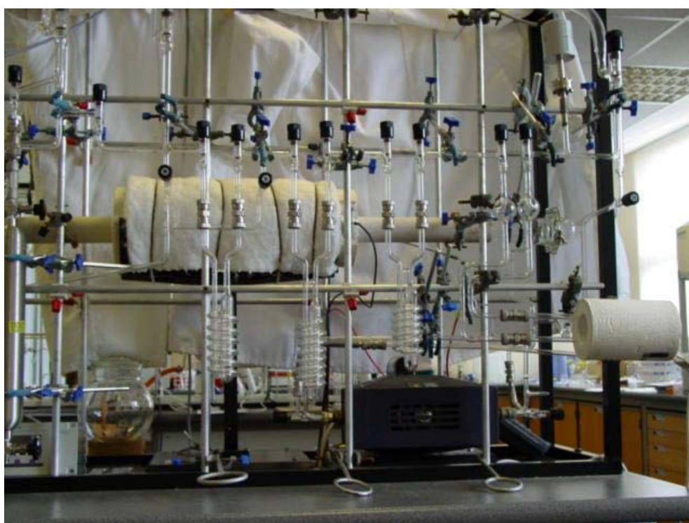
Figure 7: The combustion section of the in situ vacuum system
