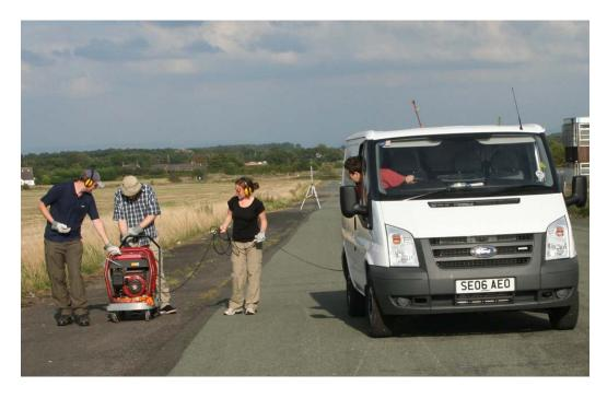
Figure 5.1: The portable instrument was housed in a van and the generator was transported on a trolley. Ethane concentration measurements were made via a sample inlet tube mounted at the top of the vehicle. Measurements of wind speed and direction were made using an anemometer (shown in the distance).
