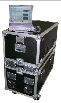
**Figure 1.** The ultra-sensitive, real-time ethane spectroscopy system developed at the University of Glasgow. The instrument with dimensions  $1 \text{ m} \times 0.5 \text{ m} \times 1 \text{ m} (L \times W \times H)$  is completely self-contained.
