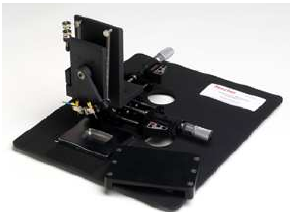
Figure 2.5: Technique for creating TMA ( www.tissue-array.org )
