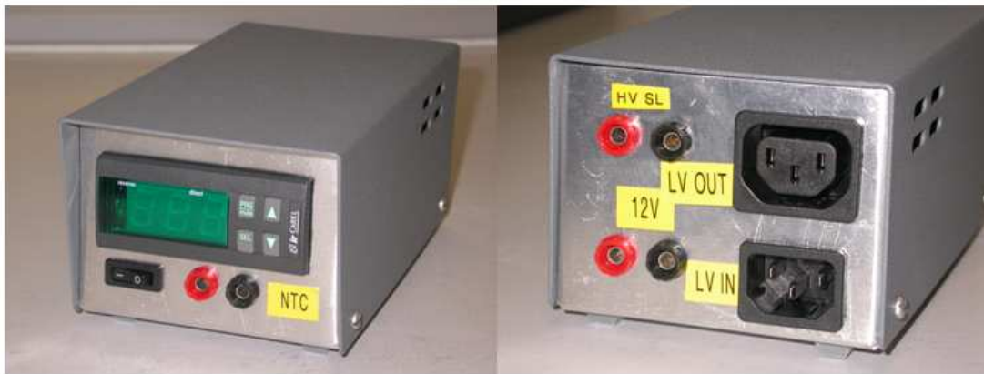
Figure 3.11: Temperature interlock schematic and pictures of the unit. The input signal was the resistance read from one NTC on the hybrid. The current temperature was shown in the front panel display. The unit used two relays to interlock both high voltage and low voltage units. On the back panel the HV safety loop and Agilent power cable were connected. In case of module overheating both connections would open and turn off the module power supplies.
