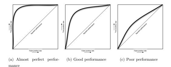
Figure B.2: Receiver operator characteristics curves for various performances.
