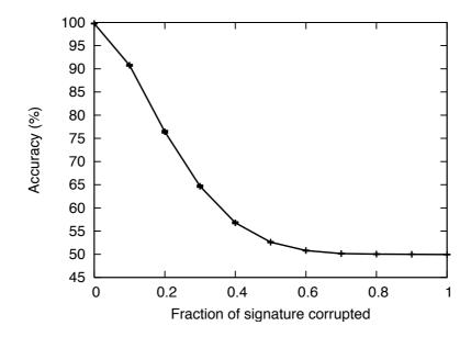
Figure 5.15: Prediction accuracy at various degrees of signature corruption. Data-to-signature ratio is 25:1.
