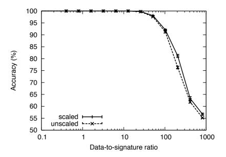
Figure 5.12: Prediction accuracy versus data-to-signature ratios for normalised (scaled) and unnormalised (unscaled) data.
