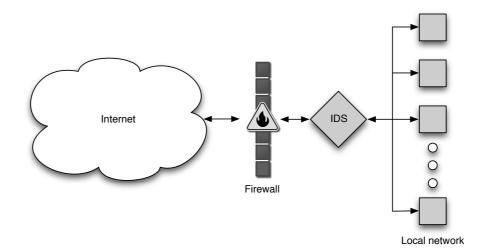
Figure 4.10: Intrusion detection systems are typically deployed behind an organisation's firewall and provide the second line of defence to all hosts on the local area network.
