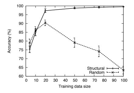
Figure 7.7: **Randomly mutated Distcc worm**. Prediction Accuracy vs training data size for classifiers trained of the randomly mutated Distcc worm. Mutation probability was 0.005 with a chunk size of 300 bytes.
