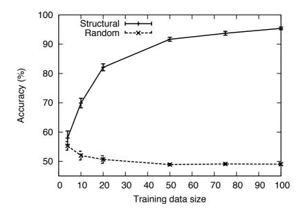
Figure 7.9: **Randomly mutated WarFTP worms**. Prediction Accuracy vs training data size for classifiers trained with generated WarFTP worm mutations. Mutation probability was 0.0001 with a chunk size of 1000 bytes.
