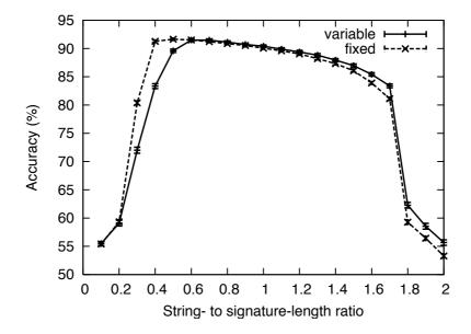
Figure 5.7: String kernel accuracy at various string-length to signature-length ratios comparing fixed and variable length strings. The data-to-signature ratio was 100:1.
