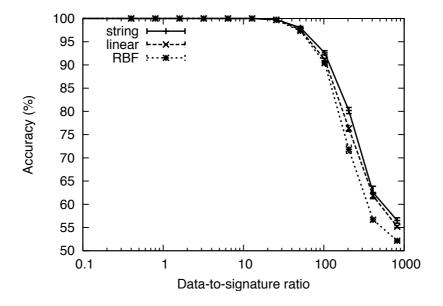
Figure 5.8: The prediction accuracy at various data-to-signature ratios for the linear, RBF, and string kernel.
