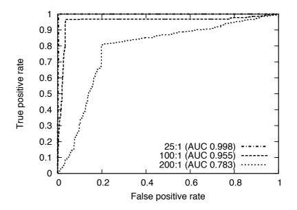
Figure 5.17: ROC curve showing the trade-off between true and false positive rates for various data-to-signature ratios.
