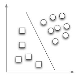
Figure 3.1: Classification involves dividing the training data by a separating hyperplane. In 2-dimensional space as in the above figure the hyperplane is a line.
