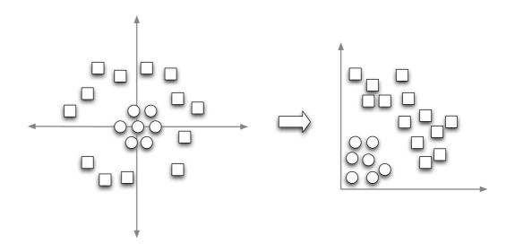
Figure 3.5: Support vector machines deal with linearly inseparable data by implicitly mapping it to a dimension where it is separable.
