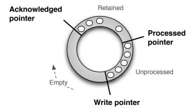
Figure 9.1: Real-time flow reassembly using a circular buffer. The circular buffer keeps track of two regions by way of three pointers: (i) a sequence of unprocessed packets, and (ii) packets that the flow analyser has requested to retain. Keeping the retained packets in the buffer as long as possible avoids spilling them to the heap.
