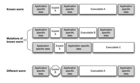
Figure 4.2: This dissertation distinguishes between mutations of the same worm and different worms by their exploit code. Worm mutations share the same exploit code, while different types of worm do not.
