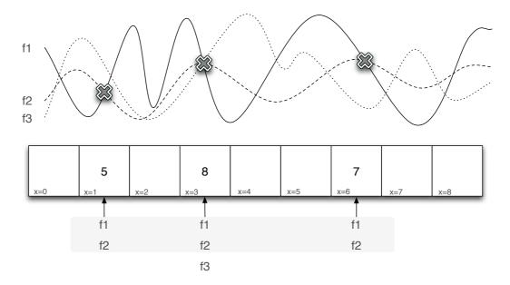
Figure 3.8: Gaussian Processes can be seen as filling a long vector where the entries hold the mean common to all Gaussian distributions in the process.
