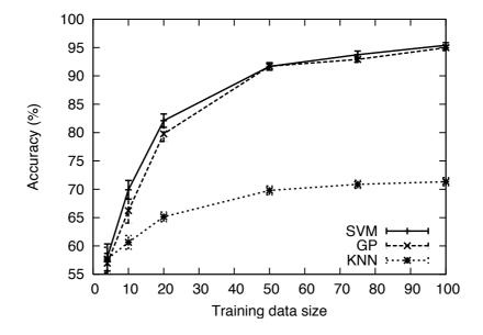
Figure 7.6: **Structurally mutated WarFTP worm**. Accuracy vs. training data size for Support Vector Machines, Gaussian Processes, and K-nearest neighbours.
