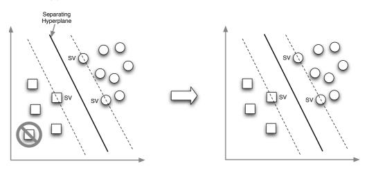
(b) Removing a vector that is not a support vector, does not affect the postion of the hyperplane.
