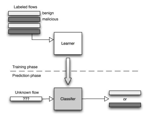
Figure 1.1: Automatically detecting worm mutations with machine learning. The learning phase is trained with network flows labelled as malicious or benign (top), producing a classifier that can distinguish between malicious and benign flows (bottom).
