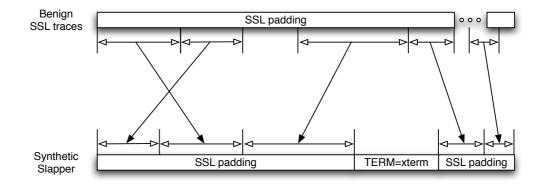
Figure 5.2: Synthetic worms loosely based on the Slapper worm consist of random-sized chunks of SSL traces used as padding.
