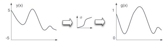
Figure 3.9: The classification function g(x) is obtained by squashing y(x) through the response function  $\sigma$
