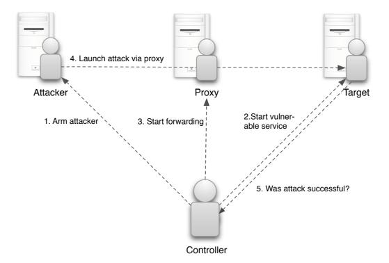
Figure 7.3: Worm testing framework. Agent interaction during an attack cycle.
