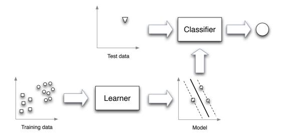
Figure 3.6: **Support Vector Machines cycle**. Training data is fed into the learner, which then builds a model that allows the classifier to classify unknown test data.
