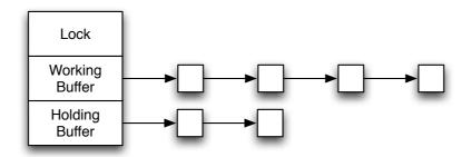
Figure 4.5: A flow consists of two packet buffers and a read-write lock. Maintaining a holding buffer for when the flow analyser examines the flow prevents packets from being discarded.
