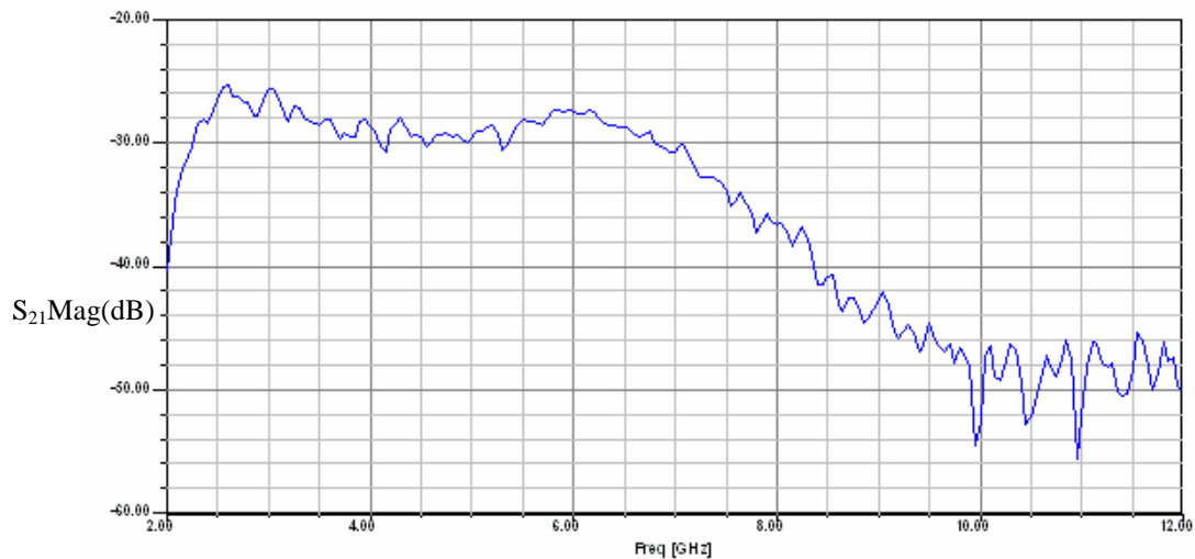
Figure 9.20. Transmission response ( S_{21} ) for CPW-fed UWB dipole with slots.
