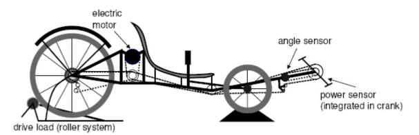
Figure 3.2: A schematic representation of the tricycle used for laboratory testing [85]
