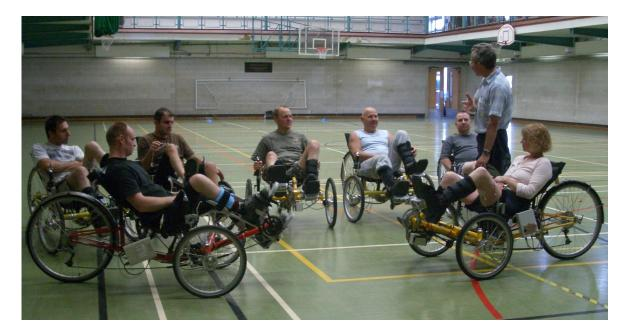
Figure 3.1: Some of the subjects preparing for an indoor sports day in Salisbury 2005. These tricycles were also used for home training purposes with the rear wheel mounted on an electronically braked cycle trainer. The stimulators can be seen attached to the frames of the tricycles in the foreground of the photograph.
