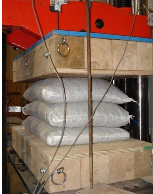
Figure 4. Earthbag specimen with loading plates on top and bottom.
