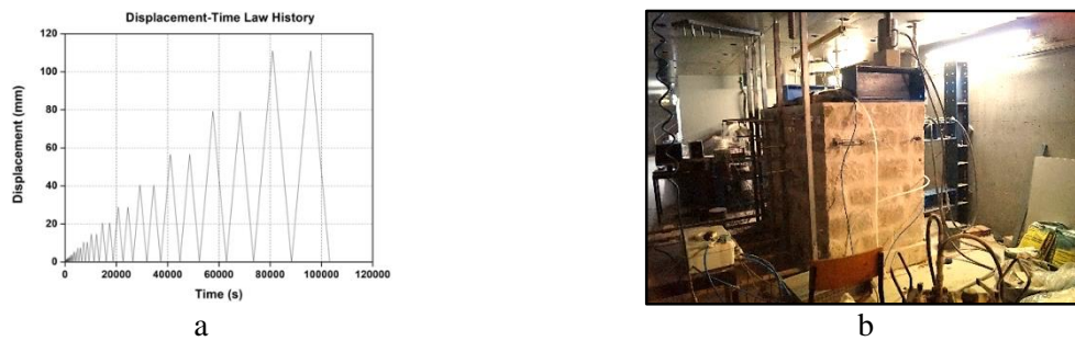
331 Figure 11 – Displacement-time law history (a); airbag pressure system (b)
