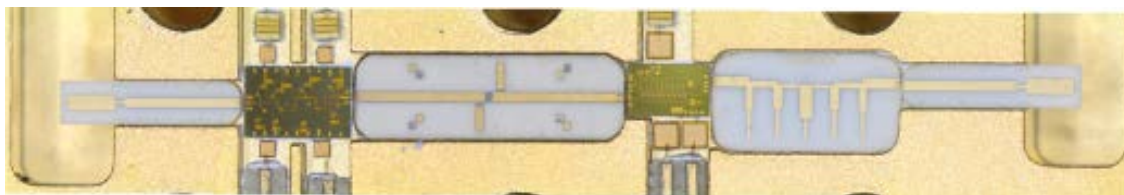
Figure 14. FGI BEM low-noise amplifier, internal view
