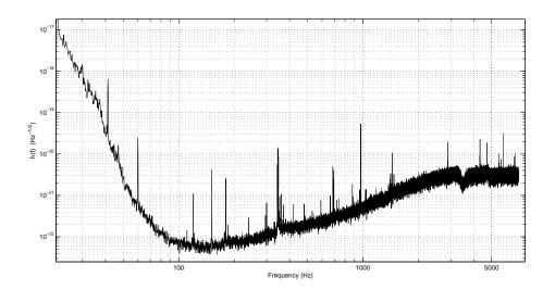
Figure 4.1: Plot showing the strain sensitivity during the S3 science run of the 4 km interferometer at LIGO Hanford Observatory as a function of frequency.
