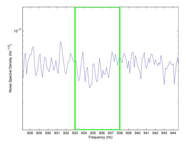
Figure 4.6: The published spectrum from LIGO Hanford 4km Observatory of strain sensitivity averaged over the S3 run, showing the frequency window which is to be searched. There are no strong lines present in this region of the spectrum, so the approximation that the band is flat is appropriate across its width, with no systematic bias toward either end.
