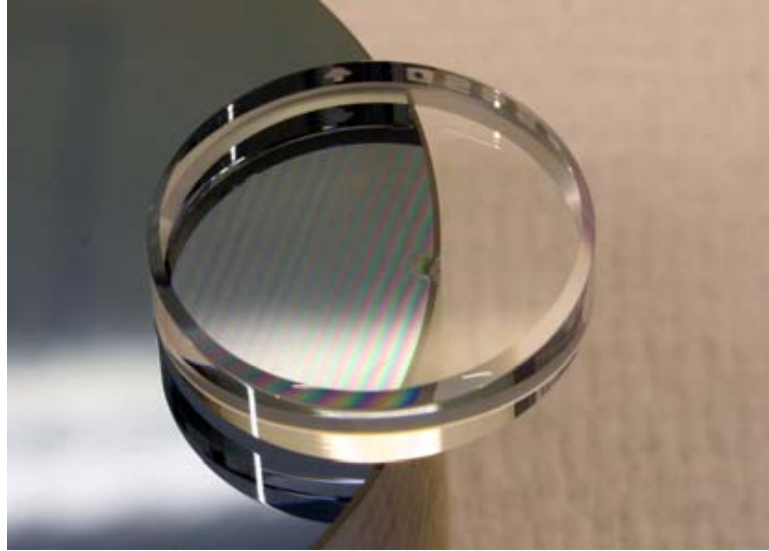
Figure 5.19: Silicon \langle 100 \rangle , 65 mm diameter and 50 mm long mass with a raised area removed, a flat polished to > \lambda/10 on top of chip to show fringes. The fringes go around the chip in a bow, indicating part of the raised area is still present.
