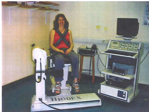
Figure 3.2: A subject seated in the dynamometer. Stabilisation straps are secured over the subject's shoulders, pelvis and thigh. The testing limb is secured to the dynamometer attachment.
