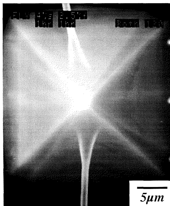
Figure 2-7 Plan view of a micromachined pyramid which has been coated using float coating. A random wrinkle has coincided with the tip in this case and could potentially affect further processing.
