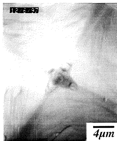
Figure 2-11 SEM of the apex of a pyramidal tip coated with 100 nm Cr. Note the star shapes region which has remained uncoated.
