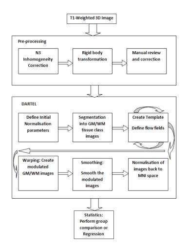
Figure 3.4: DARTEL-VBM image processing pipeline
