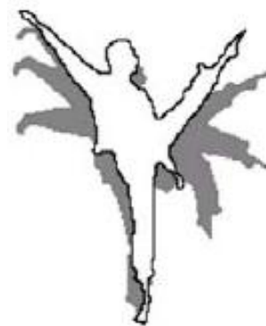
Figure 2.2: A Silhouette Motion Image (SMI) calculated over four frames. The grey area is the SMI and the dark contour is the current silhouette (Camurri, Trocca and Volpe 2003).
