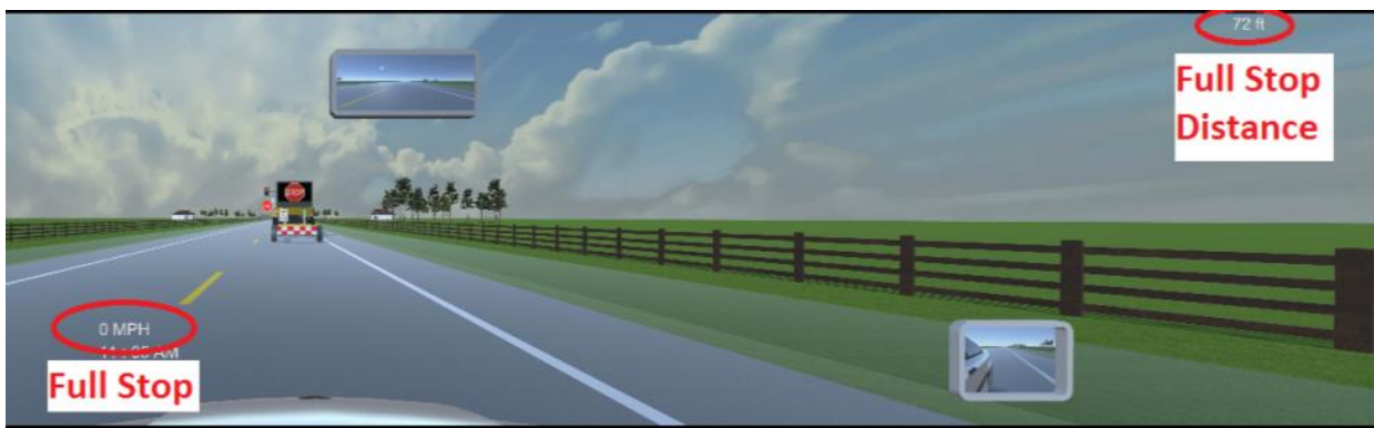
Figure 4.1.3.8 MOE 2 Example: Full Stop Distance (feet)
