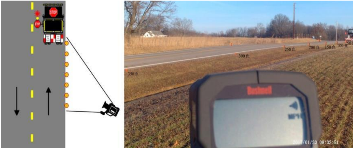
Figure 4.1.1.1 Field Study Plan of Cameras, Radar Speed Gun, and Delineators
