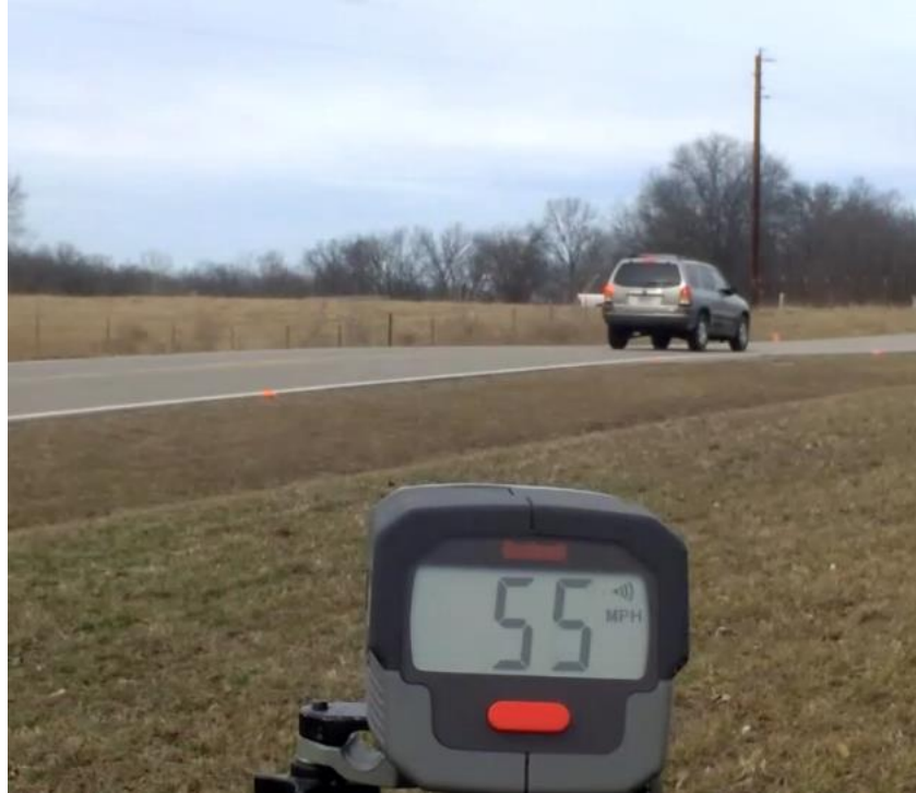
Figure 4.1.1.15 Vehicle Approaching Flagger at High Speed
