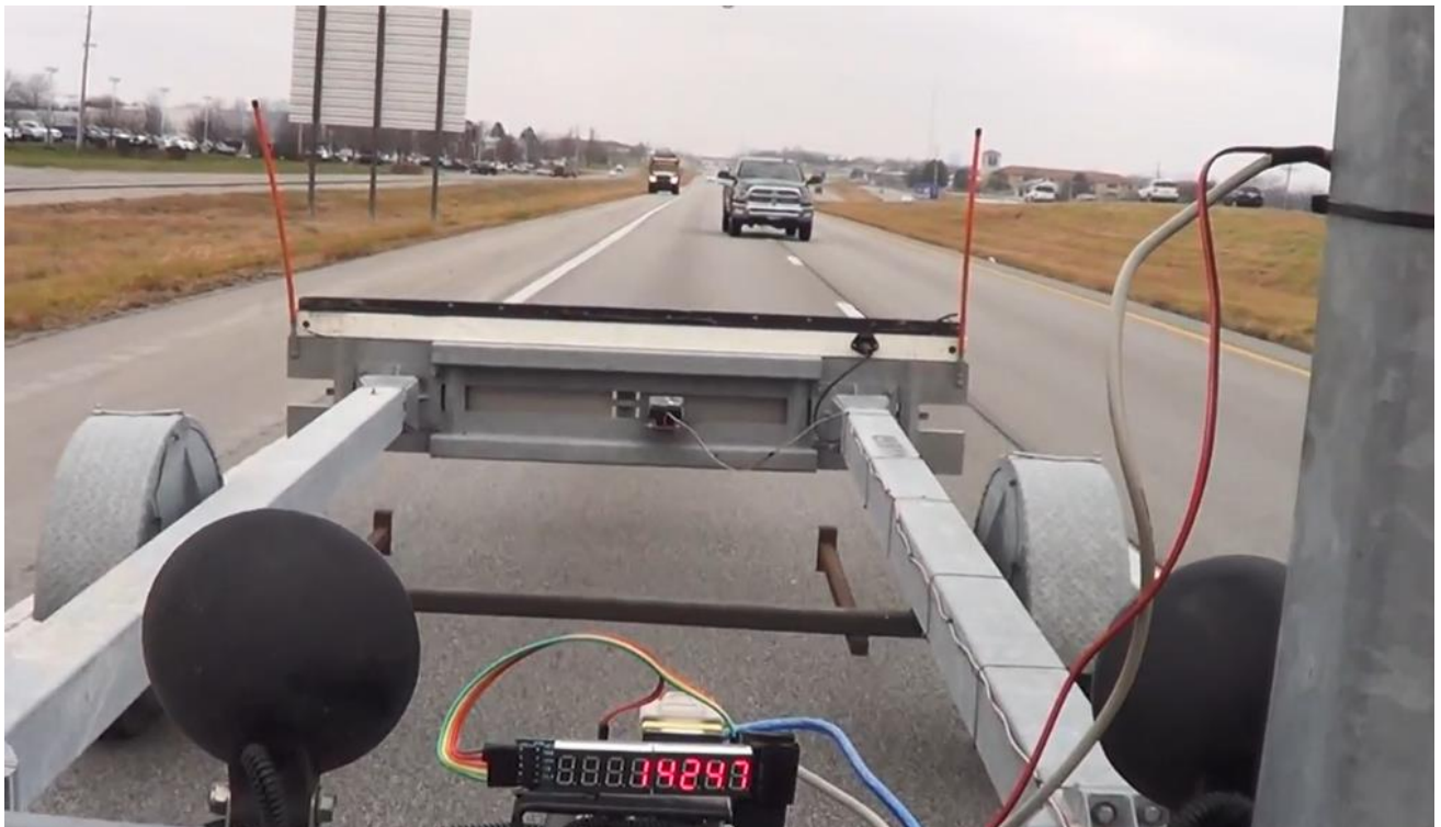
Figure 4.2.3.3 Example of LiDAR capturing distance from vehicle to rear advance TMA
